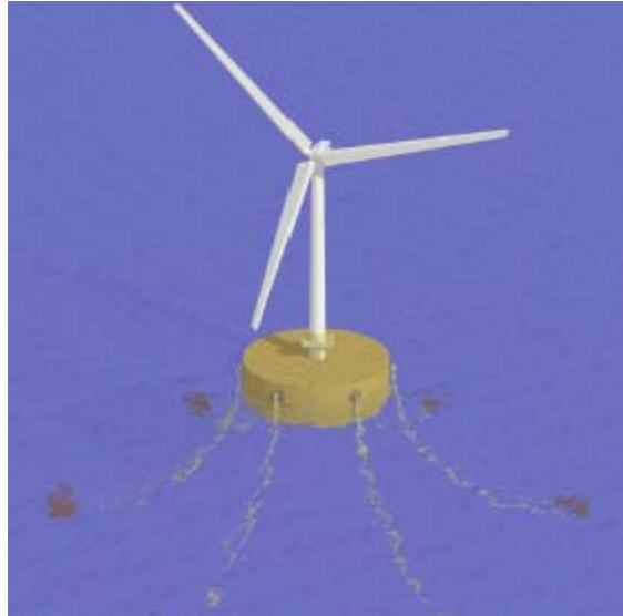
Figure 27: Single wind turbine placed on a buoy floater
