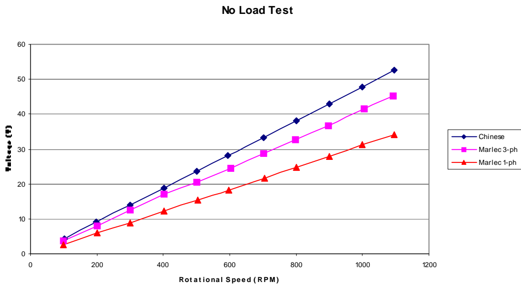
FIGURE 59 NO LOAD TEST RESULTS
