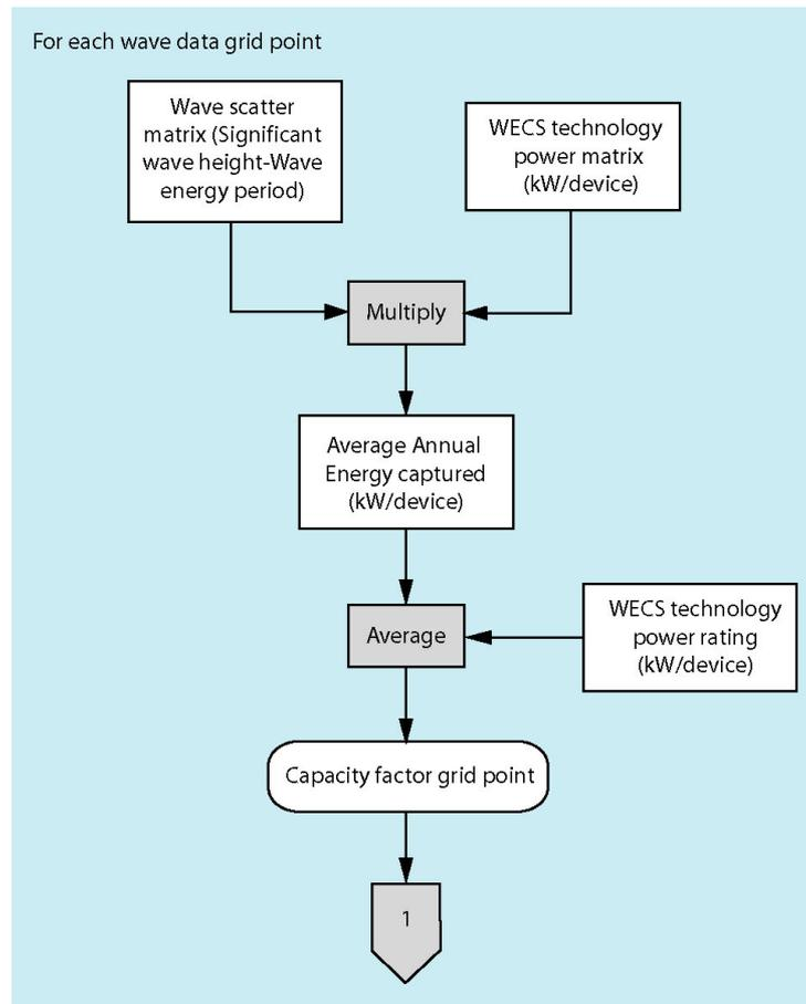
Figure 5.2: The first step in the methodology calculates the technology capacity factor for the wave device if installed at the location of the wave data.
