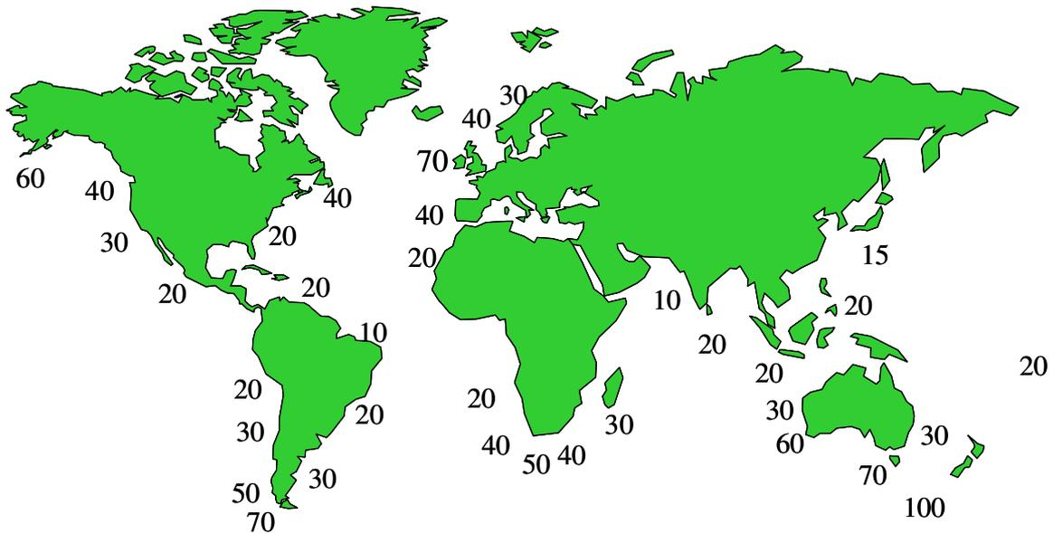
Figure 2.2: Global distribution of wave power levels in kW/m of wave crest length.
