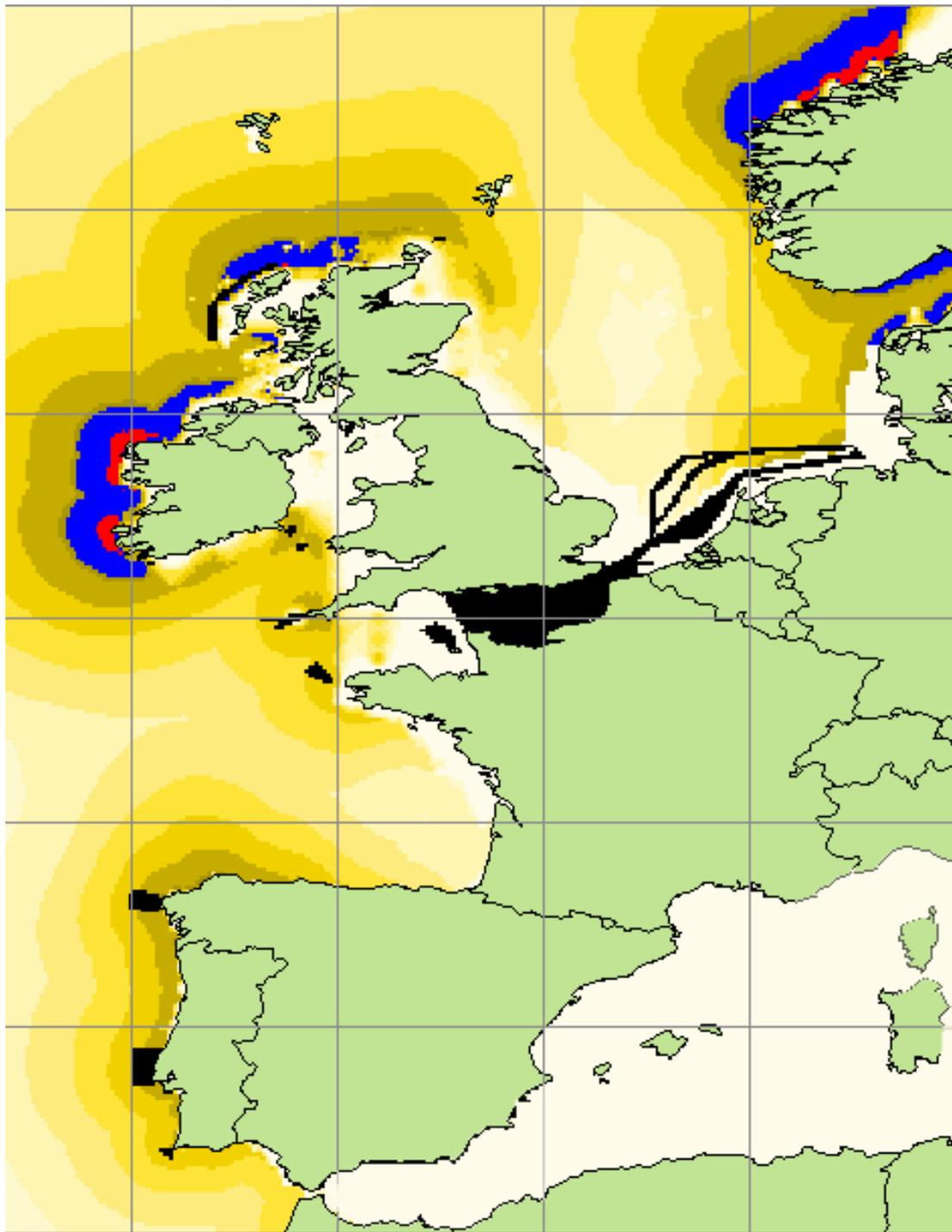
Figure 9.9: The internal rate of return GIS surface representing the estimated wave energy market for 2010 OPD WECS unit cost estimate of 750 £/kW, assuming an entry cost of 55 £/MWh. The commercially viable cells are coloured red where the internal rate of return is equal to or greater than the more realistic 13 % RRR. Both the blue and red cells indicate the equivalent market based on the optimistic return of 10 %.
