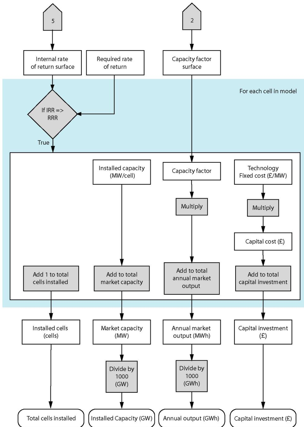
Figure 5.5: The fourth procedure in the methodology determines the number of cells within the resource model that are commercially viable if the IRR is greater than or equal to the RRR, thus identifying the economic wave energy resource and potential market.
