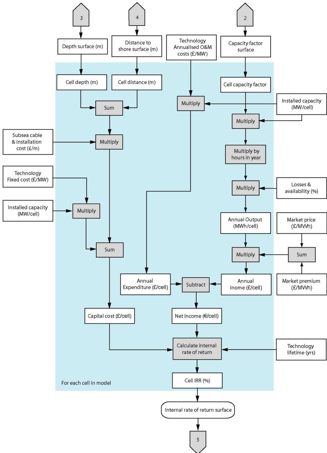
Figure 5.4: The third step in the methodology calculates the internal rate of return for potential wave energy arrays deployed in the selected area.
