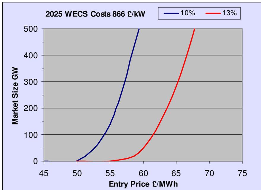
Graph 9.3: The 2025 WECS cost is estimated at 866 £/kW. The equivalent market size is plotted against the electricity entry price.
