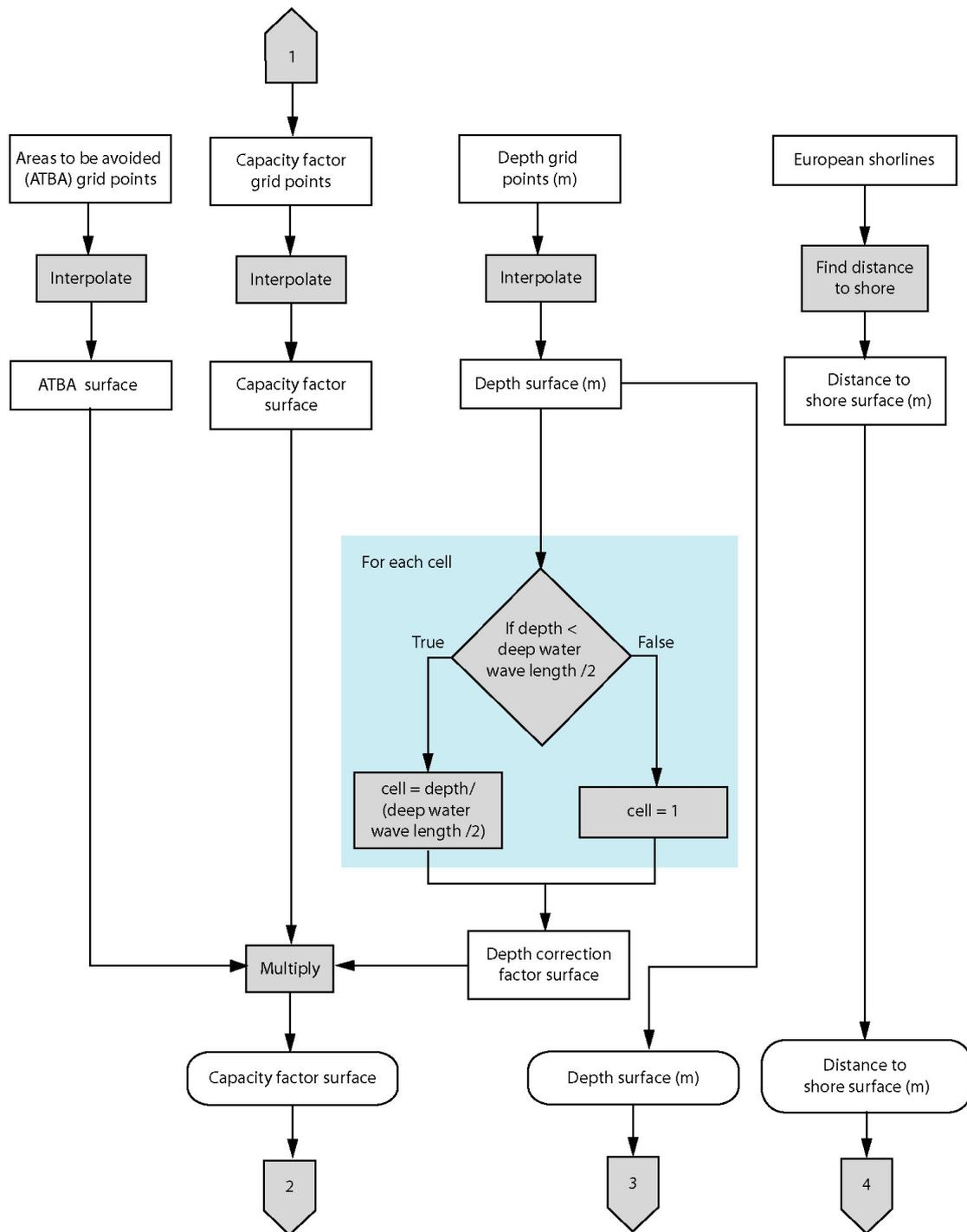
Figure 5.3: The second procedure in the methodology generates the GIS data surfaces by interpolating capacity factors and depth, and calculating the distance to shore for each cell in the resource model.
