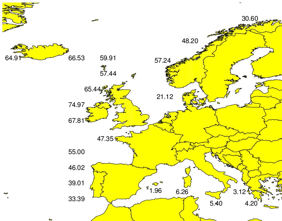
Figure 2.3: European distribution of wave power levels in kW/m of wave crest length. Source: WERATLAS. Averages are based upon on wave height and period measurements from 1987-to-1994 using the UK Met Office's European Wind-Wave Model.
