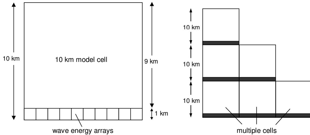
Figure 3.4: The selected device density and distance between arrays.
