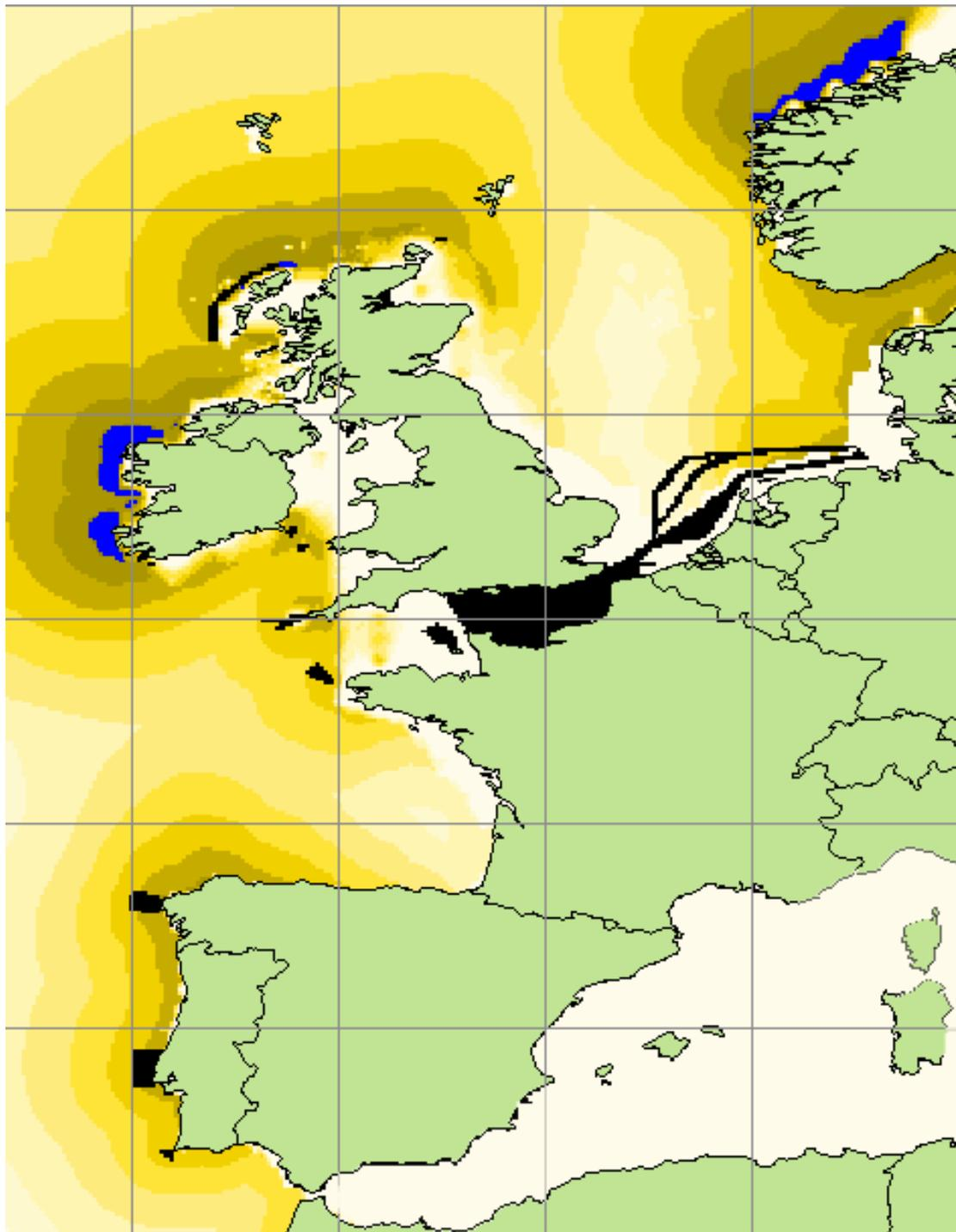
Figure 9.5: The internal rate of return GIS surface representing the economic wave energy resource based on 2025 OXERA WECS unit cost estimate of 866 £/kW, assuming an entry cost of 55 £/MWh. The commercially viable cells are coloured blue where the internal rate of return is equal to or greater than the required 10 % return.
