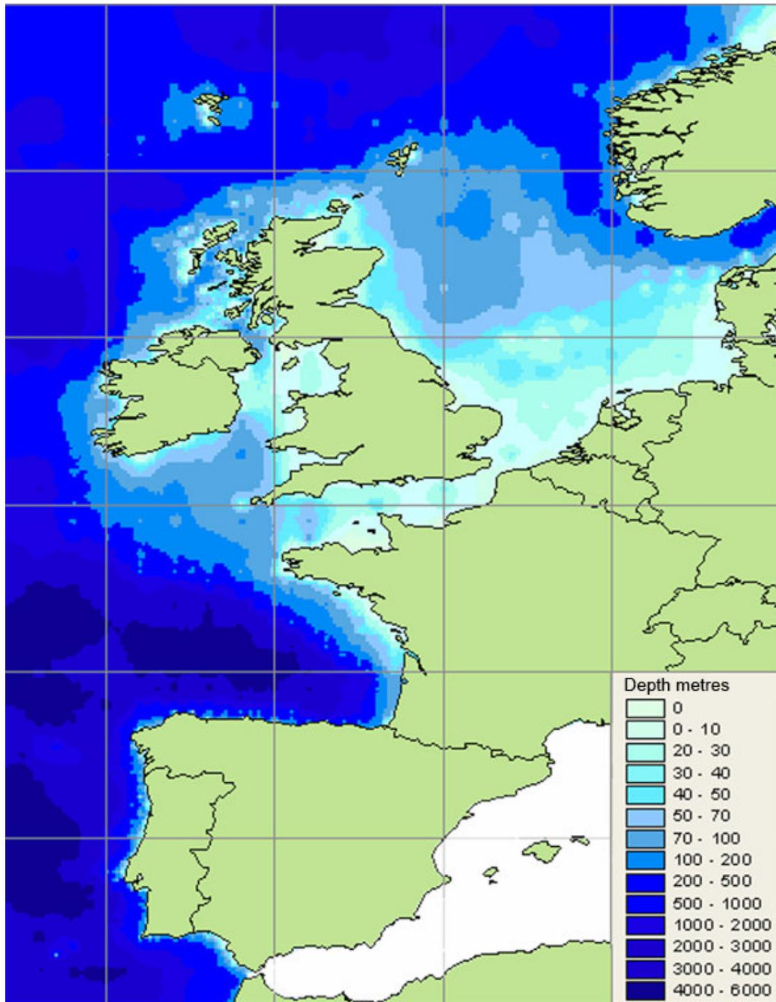
Figure 7.4: The GIS bathymetry surface, in metres, is interpolated from the gridded depth data input into the GIS model. Over 2700 depth measurements covering the Northern Atlantic Ocean and North Sea are obtained from UKHO Admiralty Charts [44]. The average depth must be calculated for each cell within the resource model, combined with the distance to shore, so that the cost of transferring the captured power onshore using submarine cable can be calculated.
