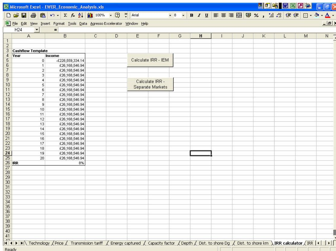
Figure 6.13: Comparing the IRR to the RRR in each cell identifies the potential market. Selecting the appropriate button initiates the Visual Basic algorithm, which automatically calculates the rate of return for each cell (using the Excel IRR function). Two different algorithms are required to calculate the IRR under the *IEM* market scenario and the *Regional* market scenario as explained in section 4.
