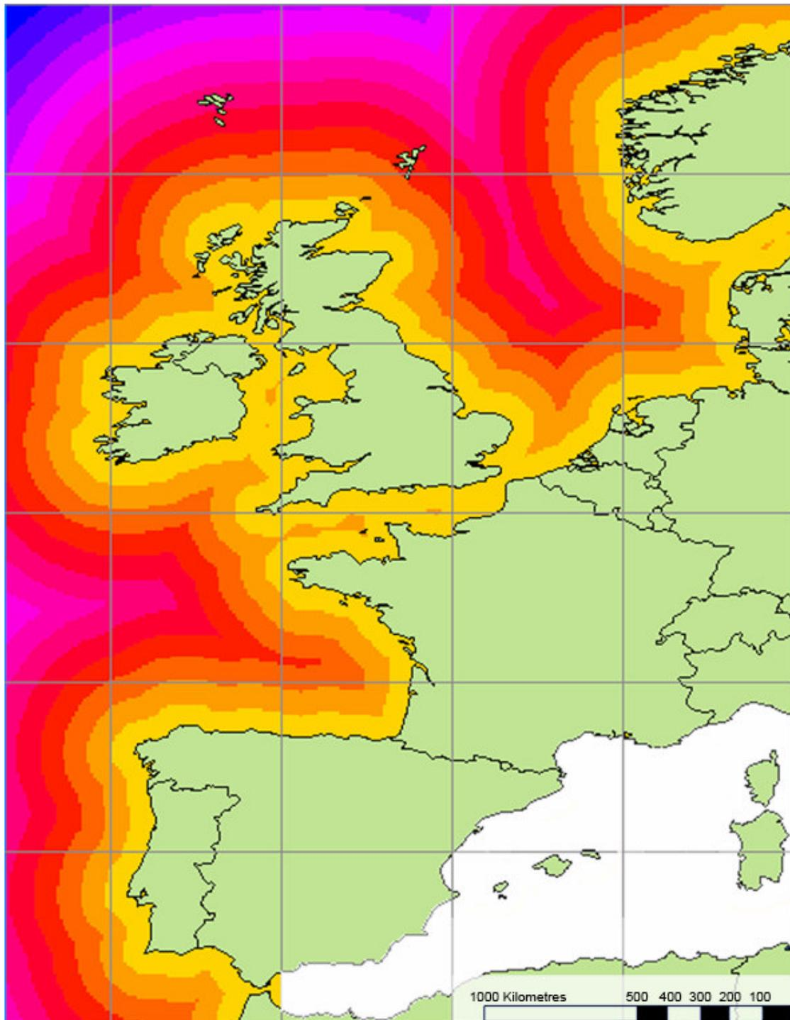
Figure 7.5: The distance to shore must be calculated for each cell within the resource model so that the cost of transferring the captured power onshore can be determined. A GIS map of Europe is input into the GIS model and the distance to the nearest shoreline for each cell is calculated in decimal degrees and then converted into metres to generate the *Distance to shore* GIS surface.
