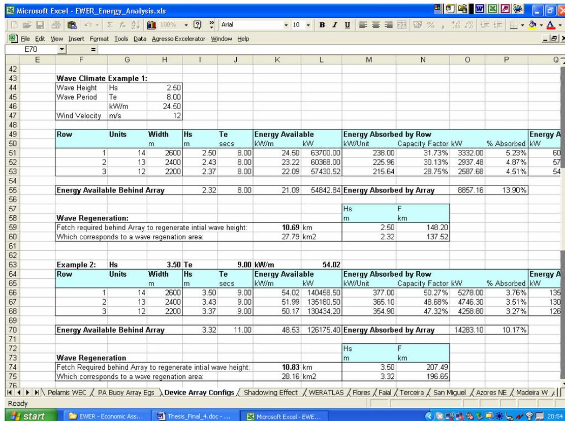
Figure 3.3: The shadowing effect is investigated for different wave conditions and assuming the OPD array layout to determine the array density to be using in the European resource assessment.
