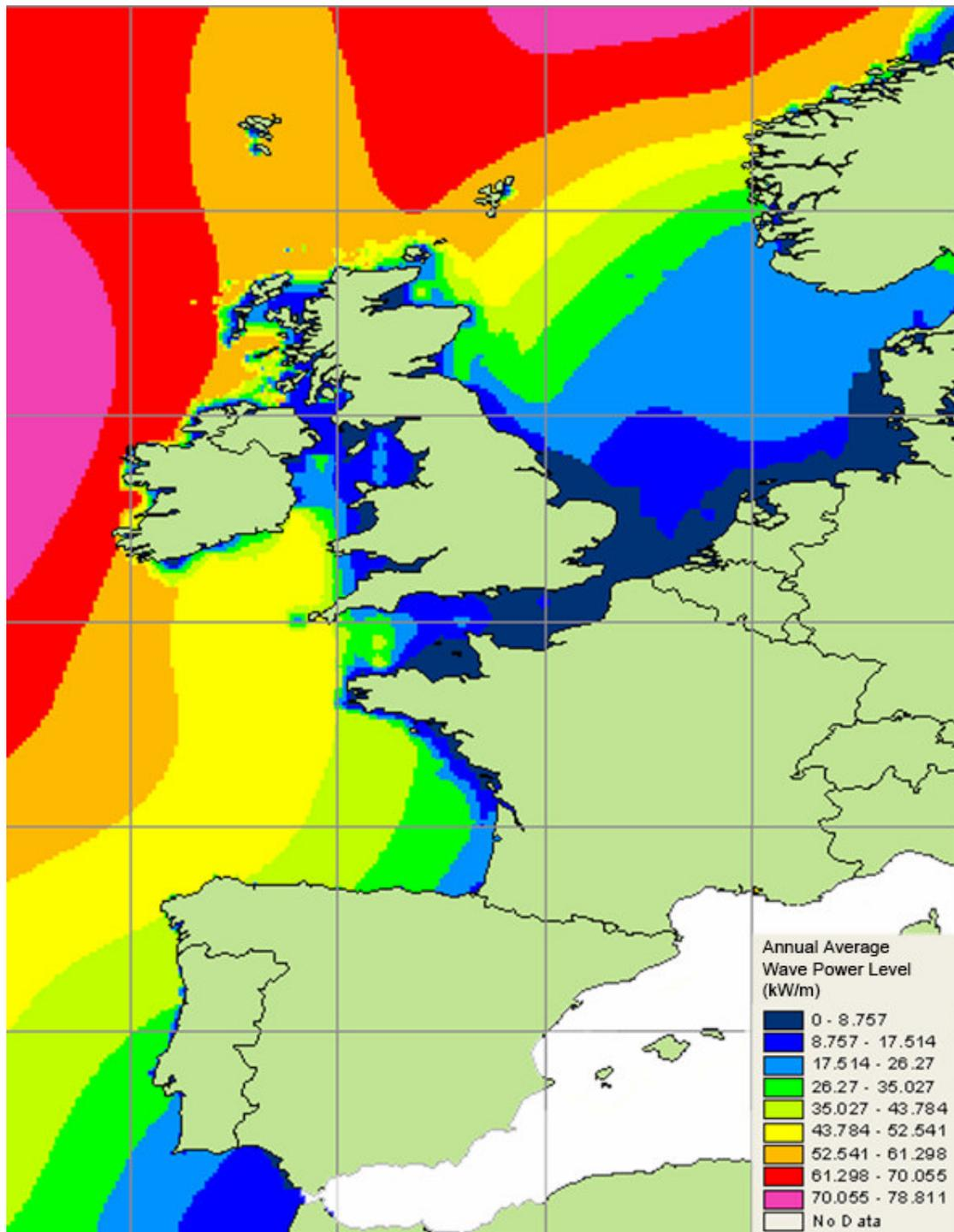
Figure 7.8: The annual average wave energy resource is interpolated from the average annual wave power levels (in kW/m) for each gridded wave data point obtained from the WERATLAS. The annual average power level available in kilowatts per metre of wave front (kW/m) is commonly used to present wave energy resource. This surface displays the distribution of the wave resource around Europe.
