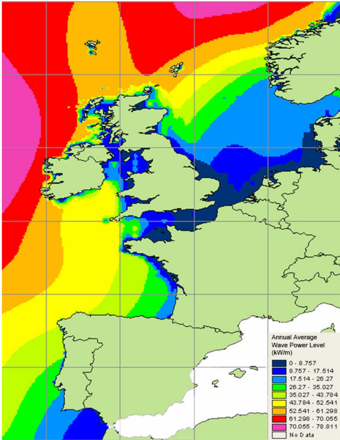
Figure C: The annual average wave energy resource is interpolated from the average annual wave power levels (in kW/m) for each gridded wave data point obtained from the WERATLAS. This surface displays the distribution of the wave resource around Europe.
