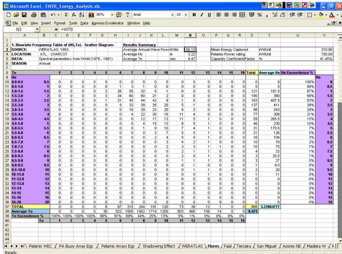
Figure B: The wave scatter diagram representing the wave conditions for a deepwater location off the Portuguese coast.
