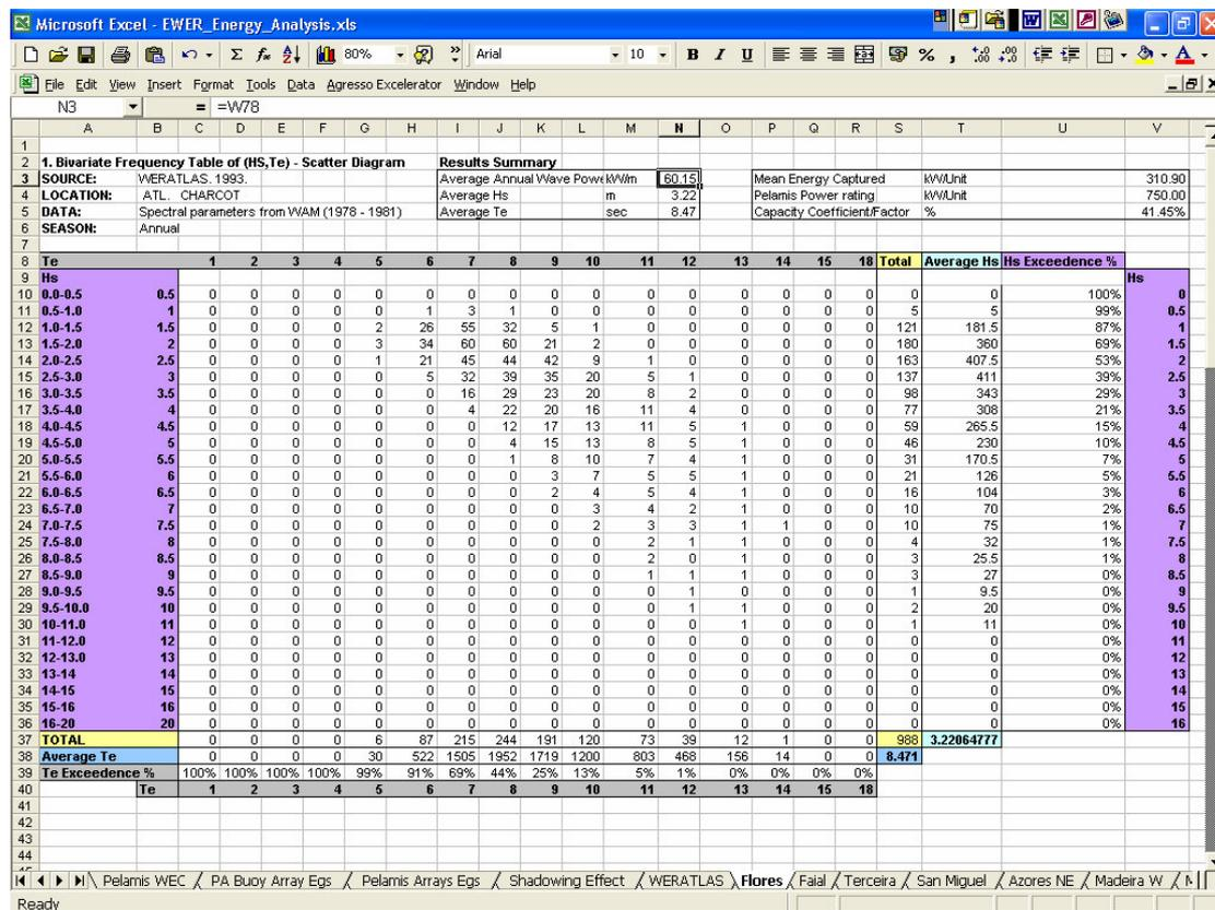
Figure 6.2: The wave scatter diagram representing the wave conditions for a deepwater location off the Portuguese coast obtained from the WERATLAS and input into the Excel model.
