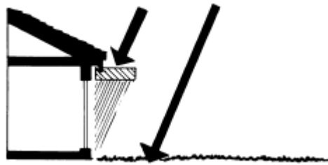
Figure 3.5 Louvered panels provide shading if the overhang is insufficient
