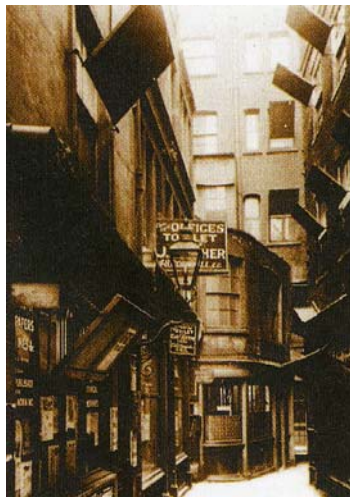
Figure 3.24 Mirrors were used to capture daylight in narrow streets in London before World War II
