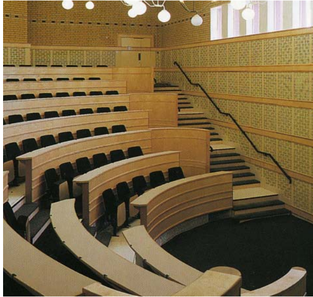
Figure 3.20 Air enters the auditorium via plena under the raked seating (Image from New Practice Case Study 102)
