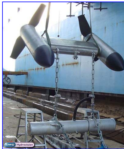
Figure 2.10 1/10 th scale TidEI tidal stream generator
