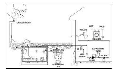
Figure 3.4.6.1: Rainwater harvesting system
