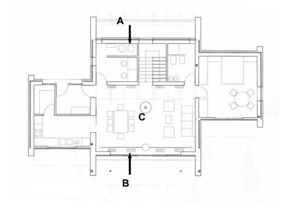
**A**: The small room where the deposit and the control for the solar collectors is located. Here there is a systems where it is possible to see the water temperature and to keep the control.
