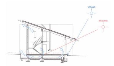
Figure 3.4.3.1: Ventilation system in the bioclimatic house of the case study. Project of the Architect Luis de Garrido
