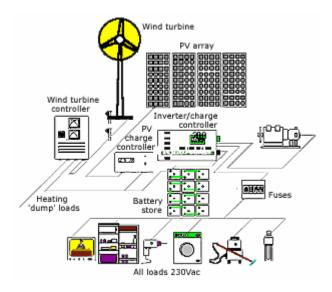
Figure 4.6: A Typical Wind, PV, Battery System
