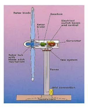
Figure 2.5: Wind Turbine Components
