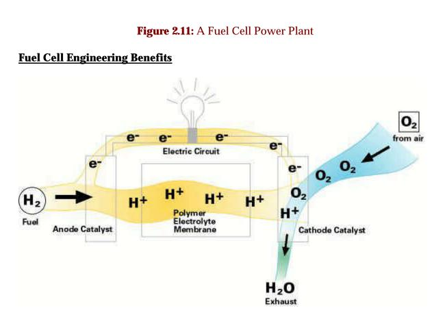
Figure 2.12: How a Fuel Cell Works
