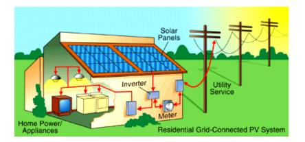
Figure 2.2: Residential Grid – Connected PV System
