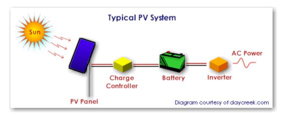
Figure 2.1: Typical PV System
