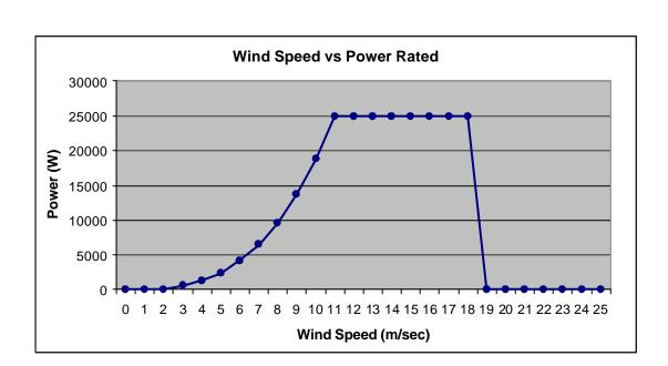
Figure 4.21: Wind Speed Vs Power Rated
