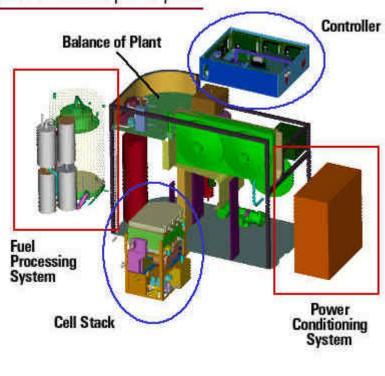
Diagram of a fuel cell power plant.
