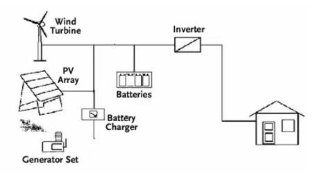
Figure 4.40: A Wind, PV, Battery System
