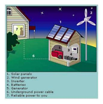
Figure 2.3: A Hybrid Wind – PV System
