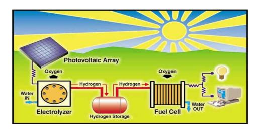
Figure 4.26: How a Renewable System Works with a Electrolyser/Fuel Cell
