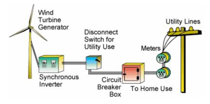
Figure 2.4: A Grid – Connected Wind Turbine
