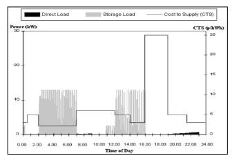
Fig: Response of the CELECT system to a cost reflective message
