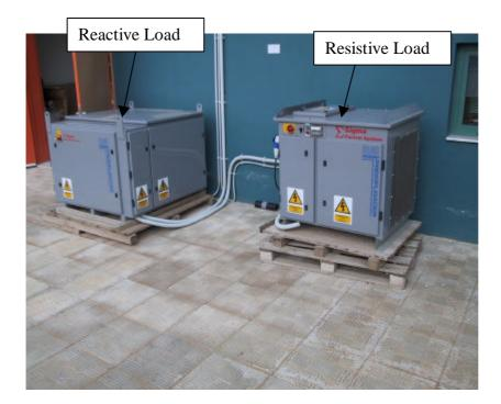
Figure 4- Resistive & Reactive Loads of the test circuits. Center for Renewable Energy Sources in Greece Department of Photovoltaic Systems
