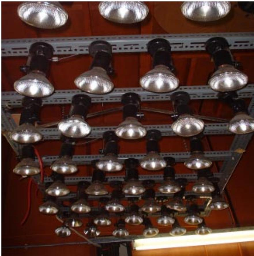
Figure 5.1 University solar simulator consists of 50 tungsten halogen's lamps, type PRA 38, manufactured by Thorn Lighting LTD
