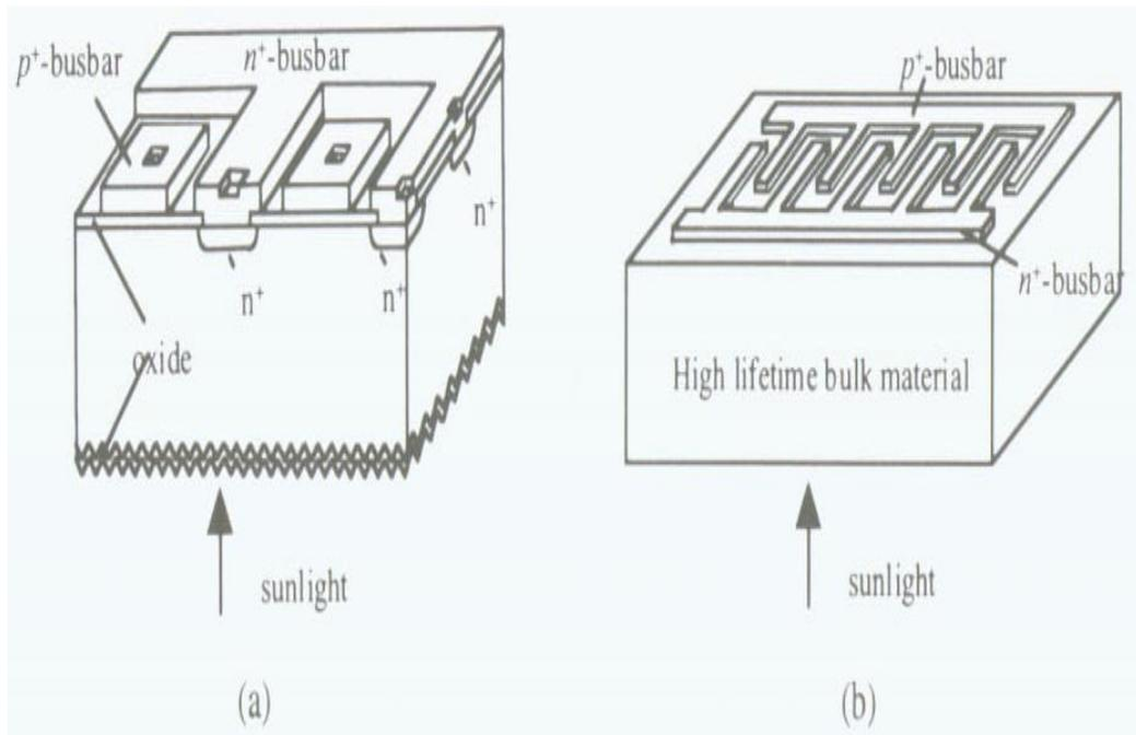
Figure (2.5) (a) backside point-contacted solar; (b) backside interdigitated solar cell.
