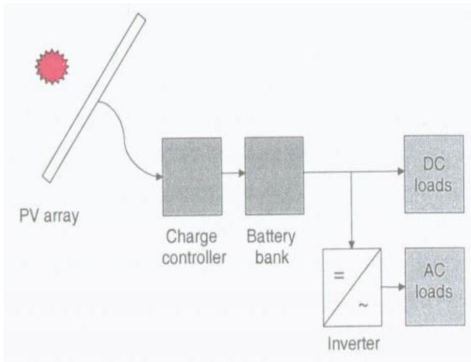
Figure 4.4 a) Schematic diagram of a stand-alone photovoltaic system.
