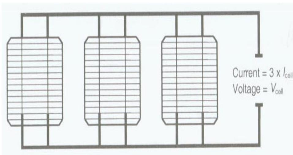
Figure 4.1 (b) parallel connections of cells
