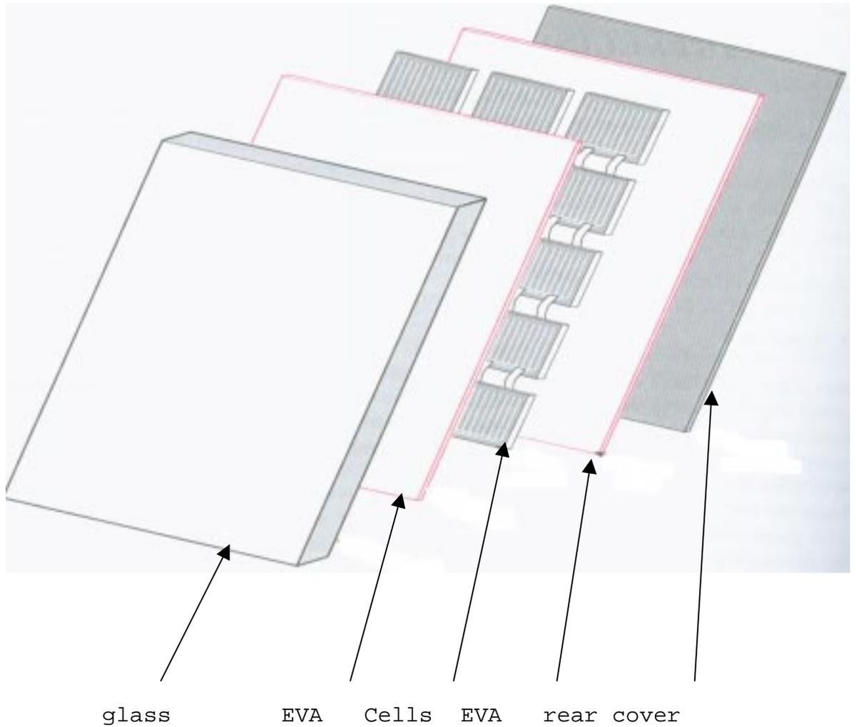
Figure (3.1) Exploded view of a standard silicon photovoltaic module. These layers laminated together under pressure at a temperature around 140-150 C where the transparent EVA (ethylene vinyl acetate) softens and binds the different layers together on cooling. Source: Green and Hansen (1998).
