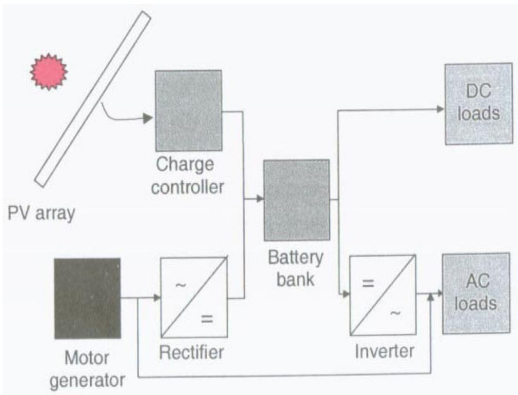
Figure 4.4 c) Schematic diagram of hybrid system incorporating a photovoltaic array and a motor generator (e.g. diesel or wind).
