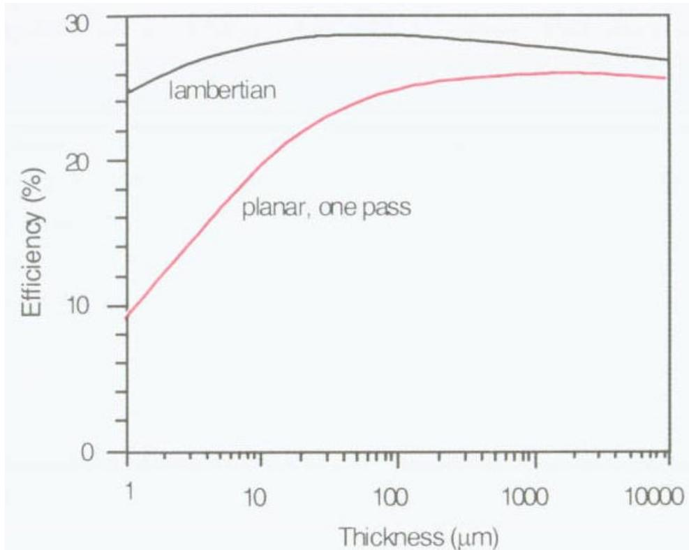
Figure (3.5) Limiting efficiency of a silicon solar cell as a function of cell thickness with and without lambertian light trapping (global AM1.5 spectrum,  $100 \text{ mW cm}^{-2}$ , 25 C). source: Green (1995).
