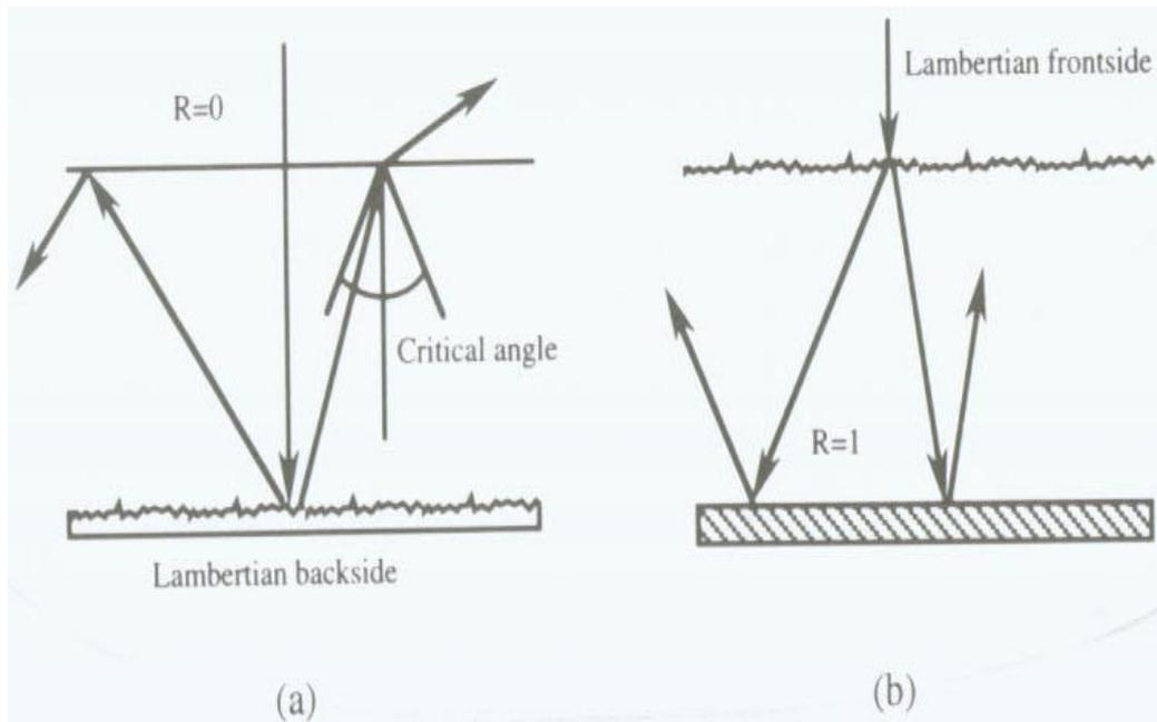
Figure (2.1) (a) Schematic of a cell with a perfect lambertian rear reflector and front surface with zero reflectance; (b) schematic of a cell with a perfect specular rear reflector and a lambertian front surface.
