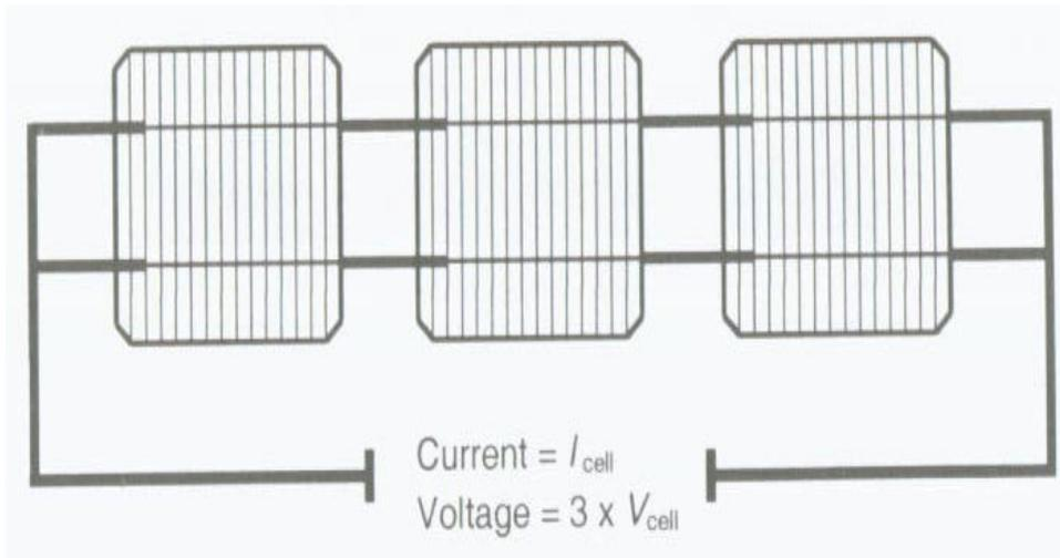
Figure 4.1 (a) Series connections of cells
