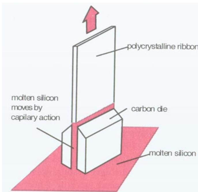
Figure (3.6) Edge-defined, film-fed growth (EFG) method. Source: Green and Hansen (1998).
