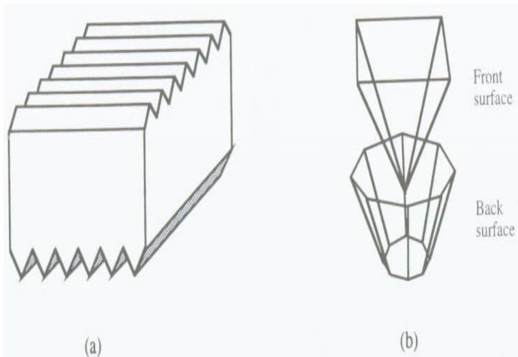
Figure (2.2) (a) Artist's view of a cell with light-trapping structures at both front- and backside. The grooves at the frontside are perpendicular to the grooves at the backside (after Green, 1995, p.104, reproduced with permission from The Centre for Photovoltaic Devices and Systems); (b) structure, proposed by Jorgensen, 1997, reproduced with permission from IEEE.)
