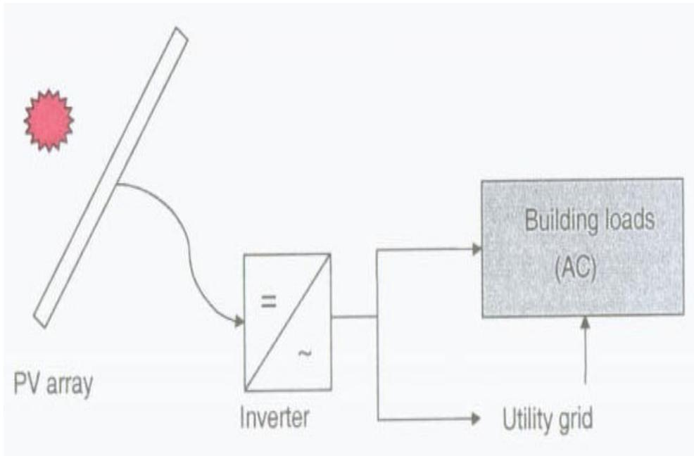
Figure 4.4 b) Schematic diagram of grid-connected photovoltaic system.
