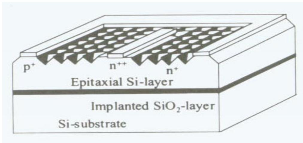
Figure (2.6) Frontside-contacted interdigitated cell (after Hebling, 1995).
