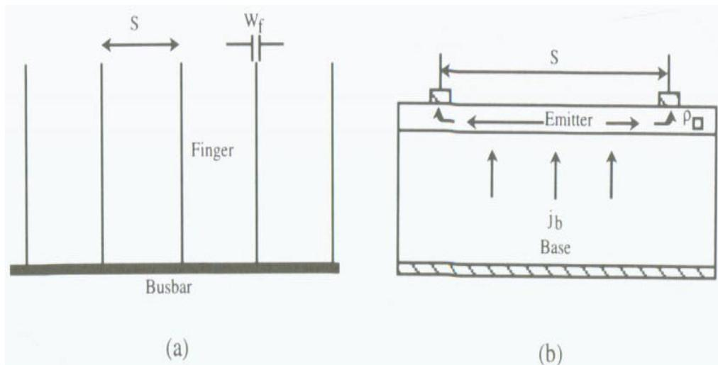
Figure (2.3) (a) Typical front contact lay-out.  $S$  is the finger spacing and  $W_f$  is the finger width. In the simple case, the finger width is constant; (b) cross section of cell showing the vertical carrier flow in the base of the cell and the horizontal majority carrier flow in the emitter.
