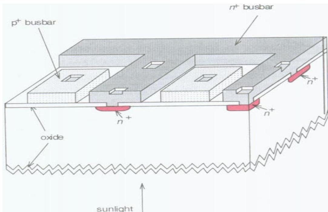
Figure (3.3) Rear point contact solar cell which demonstrated 22% efficiency in 1988 (cell rear shown uppermost). Source: Green (1995).
