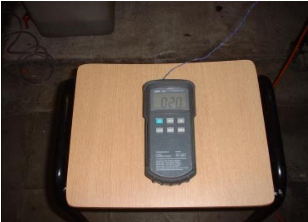
Figure (5.4) Thermometer. The range ( $-50\text{ }^{\circ}\text{C}$  to  $1300\text{ }^{\circ}\text{C}$ ) and the accuracy : ( $\pm 1\text{ }^{\circ}\text{C}$ ) for the range ( $-50\text{ }^{\circ}\text{C}$  to  $1000\text{ }^{\circ}\text{C}$ ).
