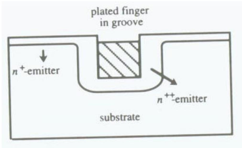
Figure (2.4) Schematic cross section of buried-contact structure.
