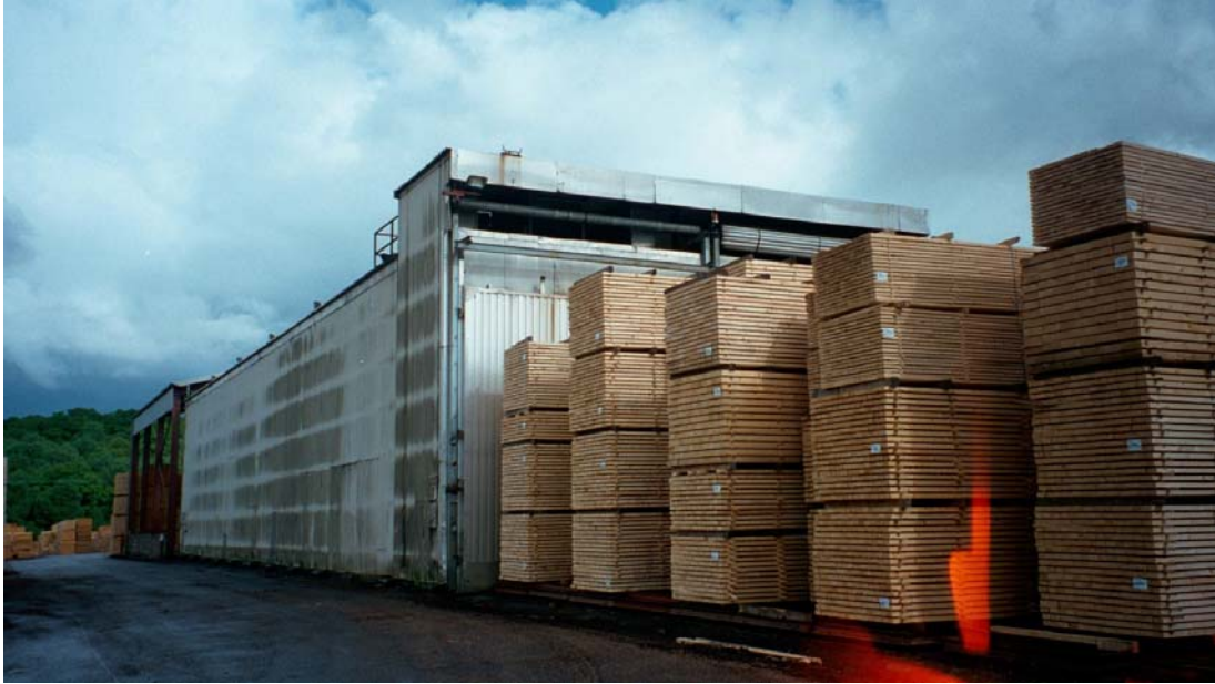
Figure 7 - Kilns 1, near, and 2, far, at the Kilmallie site, with loaded bogies waiting to enter.
