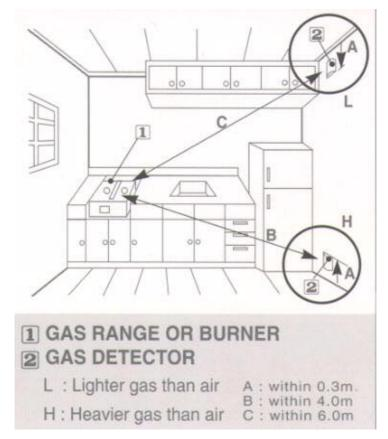
Figure 3.2.2, Typical positions for installing gas detection sensors (exact distance may vary dependant on the sensor design)
