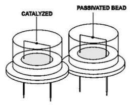
Figure 3.3.1.1, Catalytic Bead Sensor
