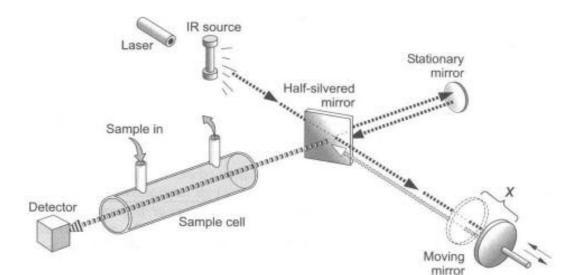
Figure 3.3.4.1, Basic Fourier Transform Infrared spectrometer
