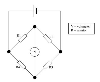
Figure 3.3.1.2, Typical Wheatstone Bridge Circuit
