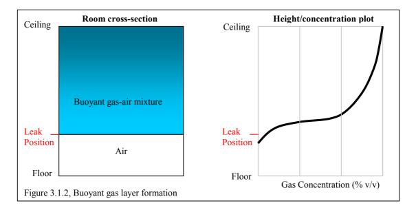
The above diagrams illustrate the general concentration profiles when gases, both lighter and heavier than air, are released into an enclosure. In order to apply the gas leak early warning system to residential buildings, it is necessary to understand the actual concentration profile of natural gas when it is released into a room since it is the primary source of gas used in UK homes.
