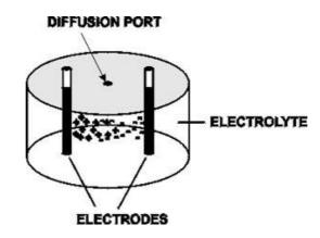
Figure 3.3.3.1, Electrochemical Sensor
