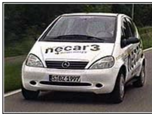
A Mercedes test vehicle that runs on fuel cell technology
