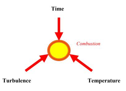
Fig. 19: The Three 'T's' of Combustion [19]
