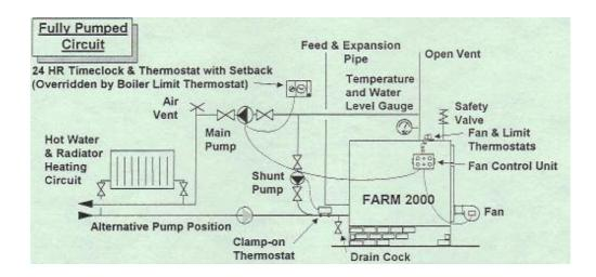
Fig.39: Woodchip boiler ('Farm 2000' model) connected into a Fully Pumped circuit
