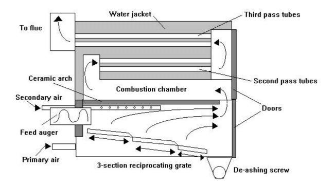
Fig. 37: The Inclined Grate design [18]
