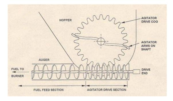
Fig. 32(c): The fuel feed system [23]
