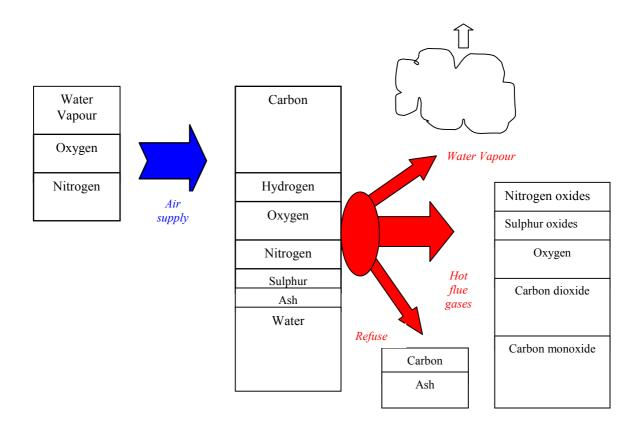
Fig.22: Simplified model of combustion balance [21]
