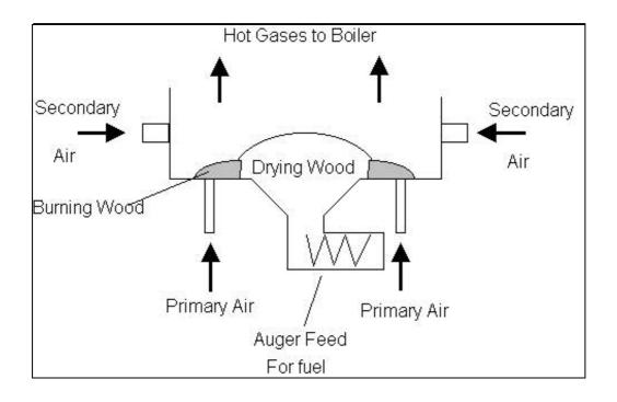
Fig. 33: The Underfeed Stoker arrangement [18]
