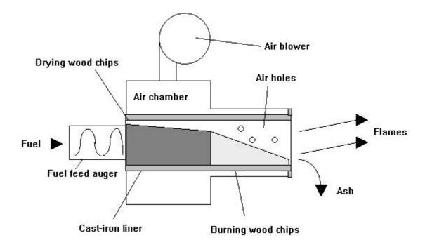
Fig. 35: The Stoker-burner layout [18]
