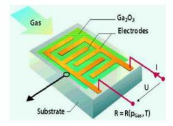
Figure 4.3 A typical gas sensor
