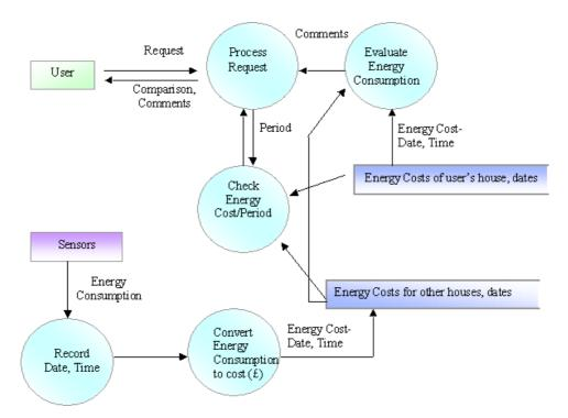
Figure 4.7 Data flow diagram for energy cost comparison
