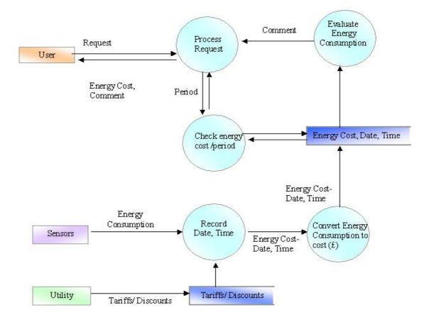
Figure 4.6 Data flow diagram for energy cost
