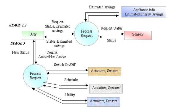
Figure 4.9 Data flow diagram for control operation of appliances
