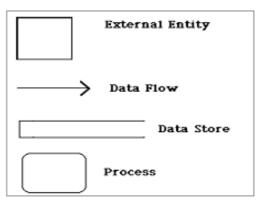
**Figure 4.4** Basic notations of the Data Flow Diagrams
