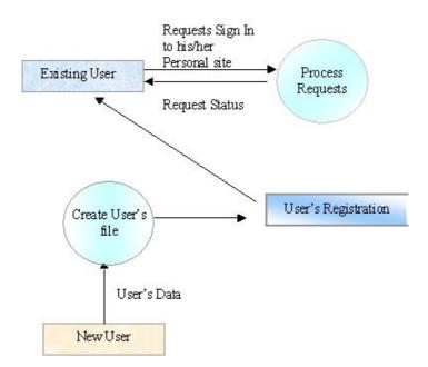
Figure 4.5 Data flow diagram for Authentication
