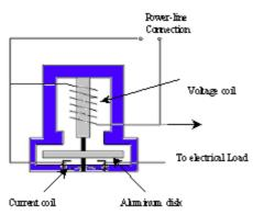
Figure 4.1 KWh meter
