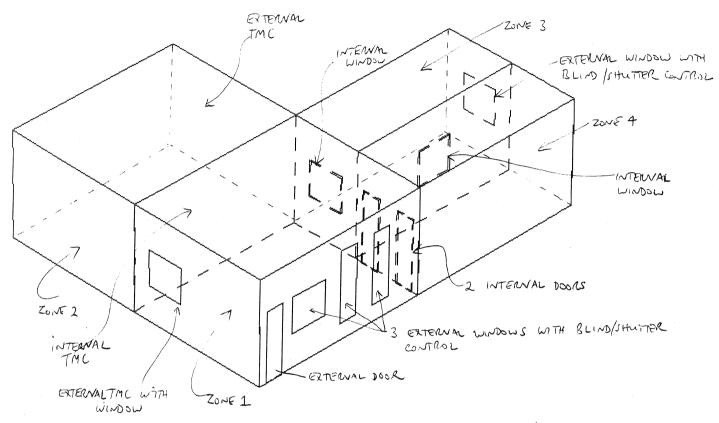
The model contains internal and external windows, TMCs and doors, and blind/shutter control of windows. For this exercise, blind/shutter control of TMCs was not used, in order that the predictions of the simulations with the old and new solar routines could be compared.
