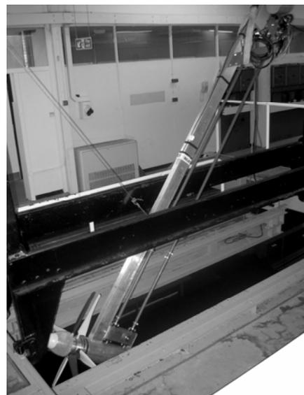
Figure 9: The test rig raised out of the tank and on the carriage.
