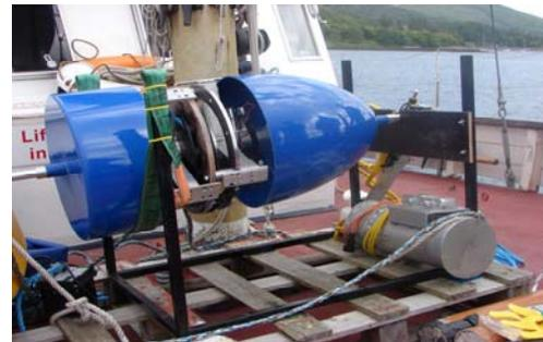
Figure 19: Generator location within the turbine nacelle.
