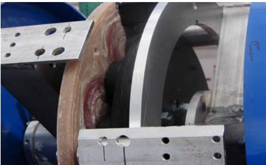
Figure 18: Encapsulated coils and permanent magnets of the contra-rotating axial flux generator.
