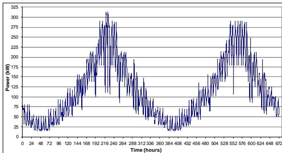
Figure 4: Fluctuations in power outputs between spring and neap tides.
