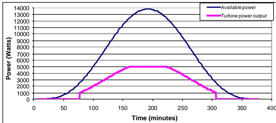
Figure 1: Turbine output relative to available power.
