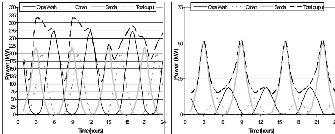
Figure 3: Site and aggregate power output for a 10m diameter tidal turbine in spring and neap tides.
