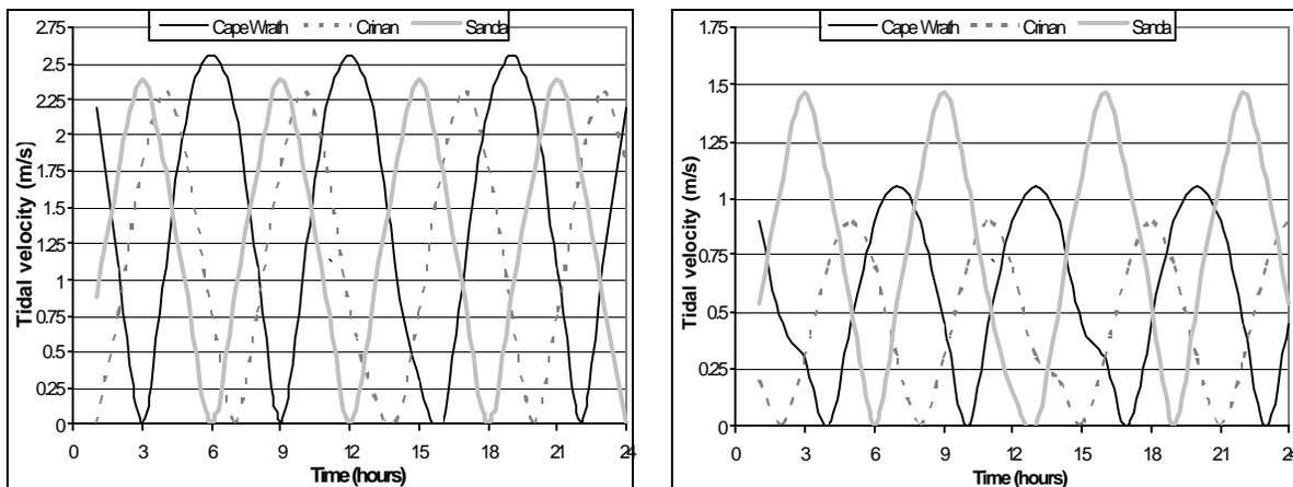
Figure 2: Spring and neap tide velocities at three sites on the West coast of Scotland.
