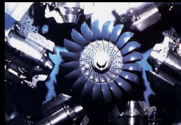
A 6-jet Pelton wheel, rated at 122 MW under a head of 650 m; Aos River, Greece
