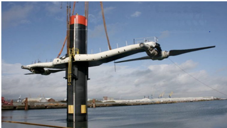
1.2 MW twin-rotor turbine, now installed in Strangford Lough, N Ireland
