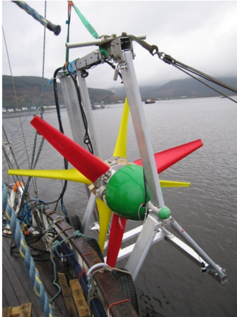
2.5 m diameter contra-rotating horizontal-axis turbine
