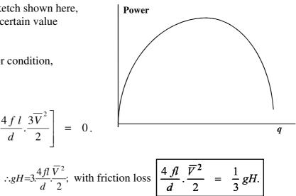
Thus the energy available at the end of the pipe =  $\frac{2}{3}gH$  and the transmission efficiency,  $\eta_{tr}$ , for the pipeline is defined as
