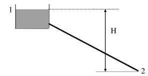
From the free surface in the reservoir to the pipe exit, the energy equation is
