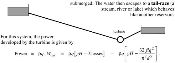
For a given system, there is a maximum power which can be made available to the turbines, its value depending on H, f, l and d.
