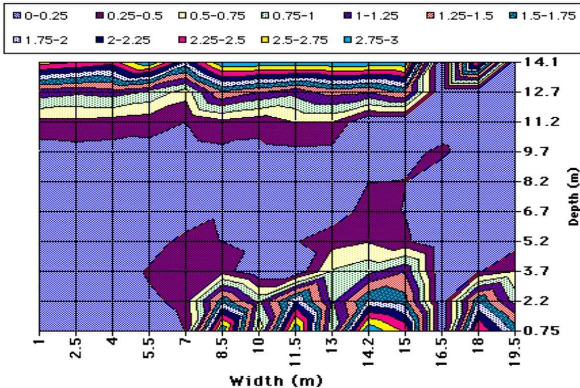
Figure 5: Daylight factors, Base case.
