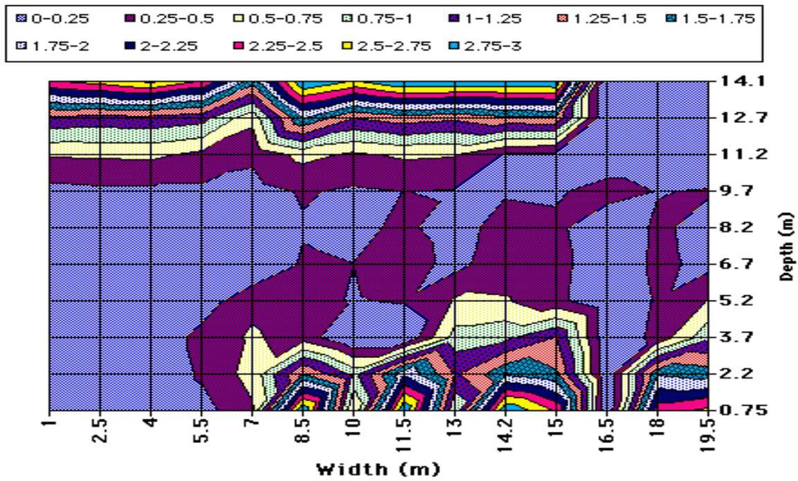
Figure 7: Daylight factors, modified interior design case.
