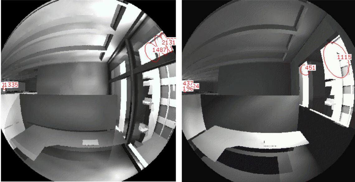
Figure 6: Comparison of glare sources in Base and Reference cases.
