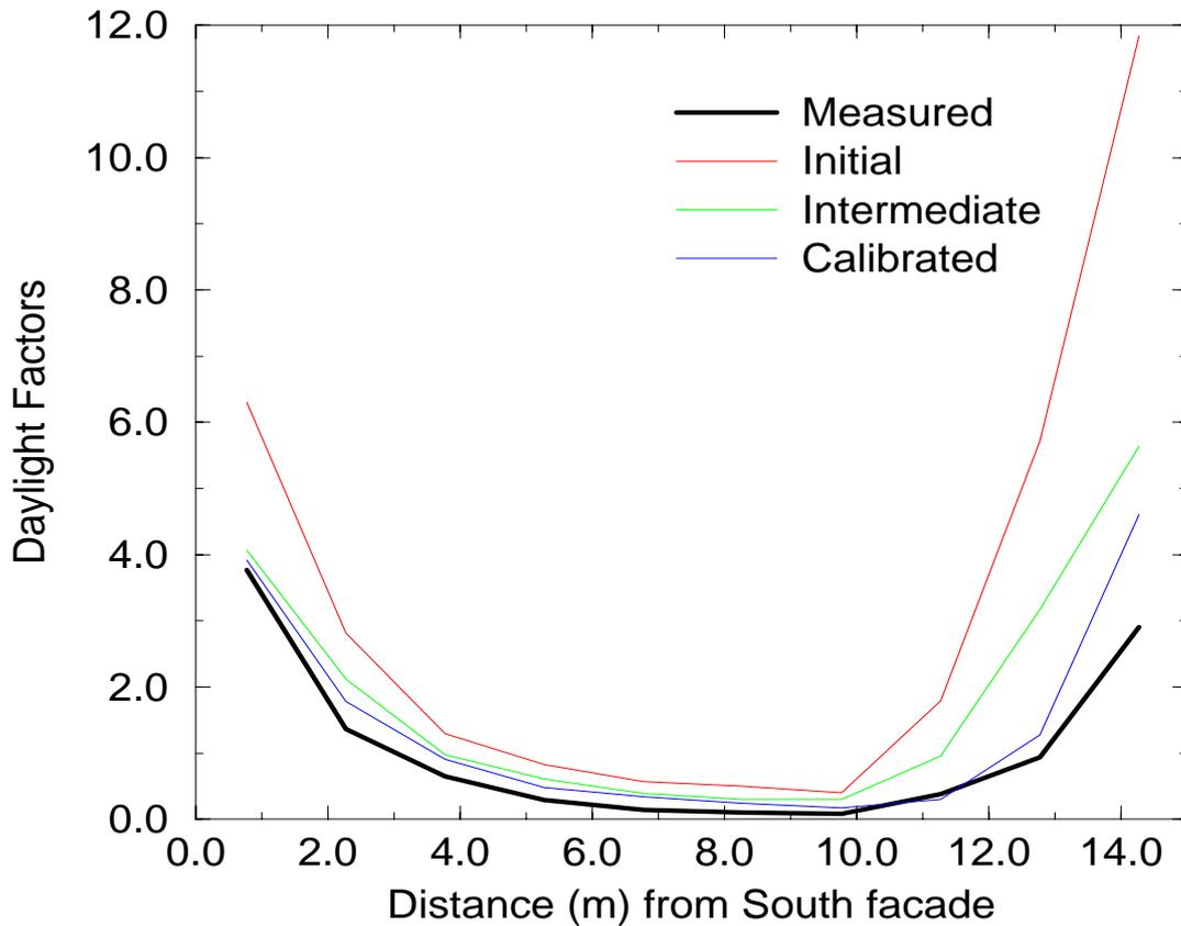
Figure 4: Daylight factors, base case model.
